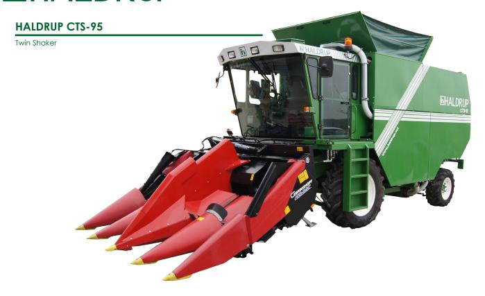
The main goal by designing the Twin Combine was to save money for the user. The goal was achieved by reducing the harvesting and analyse costs with approximately  $5 \in \text{plot}$  by reducing labour, analyse, fuel and machine costs. With the same combine you harvest simultaneously 2 plots but are using only 1 infra-red analyser, 1 computer and 2 operators.
