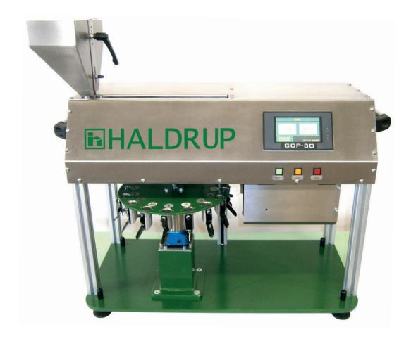
The HALDRUP GCP-30 Grain counter and filling machine counts seeds with the greatest precision and at high speed. The number of bags that the seeds are packed into can be set individually.
