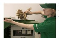
Over the feeding table, the material is supplied to the treshing drum.
